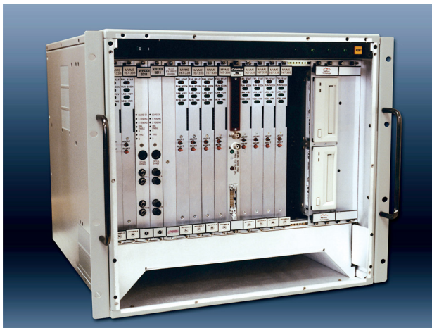
Figure 8. The LAU concept provides both physical independence as well as functional and physical adaptation to particular interface and integration needs. While operating within the overall SSDS integration and broadcast information-oriented architecture, LAU components can support processors, languages, functions, and physical interfaces that are unique to a particular interface. This prototype LAU consists of a commercial VME card cage populated with LAN interfaces, device interfaces, application single-board computers, and tape drives.
