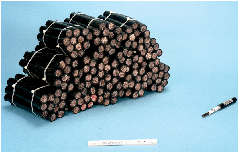
Figure 9. The 144 copper cables for CDS parallel channels on the left are compared with a single fiber-optic cable containing 144 individual glass fibers. The change in physical media, resulting in a potential cable plant weight reduction from 35.3 to 0.05 lb/ft, was only part of the technology challenge. To exploit fiber optics, an evolution in equipment interfaces was also required.
