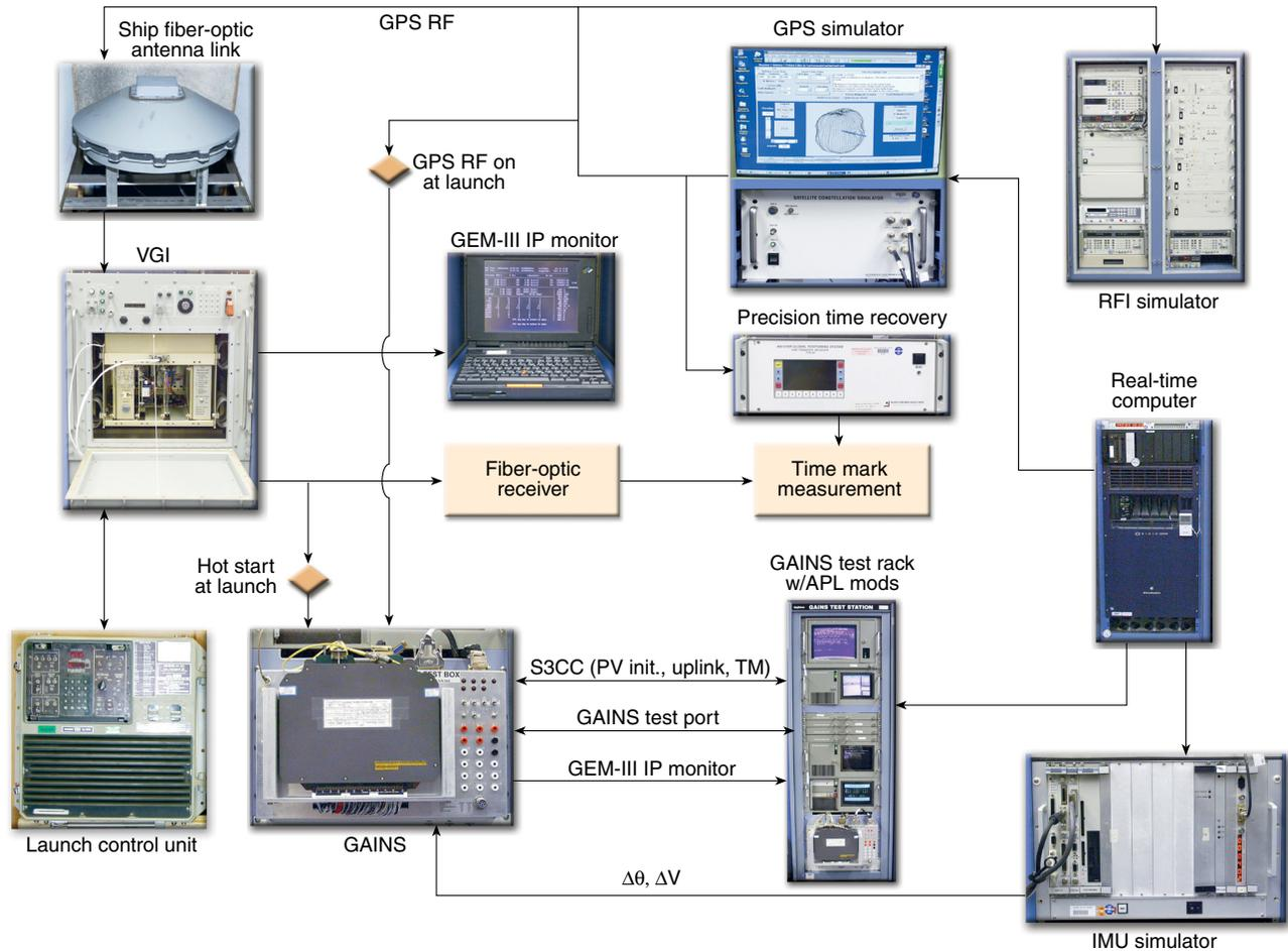
Figure 8. NAVSIL VGI hot start and GAINS test configuration.
