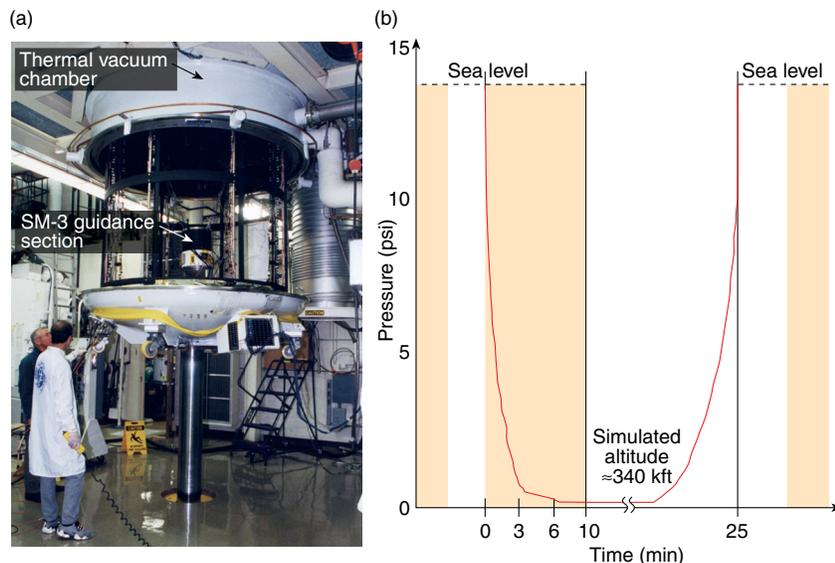
**Figure 10.** The SM-3 guidance section (a) under test in the APL Space Department's thermal vacuum chamber and (b) pressure profile during simulated high-altitude testing (shaded regions indicate time when guidance section was powered).
