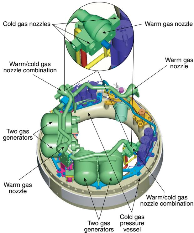
**Figure 4.** Hybrid Warm/Cold Gas Attitude Control System.
