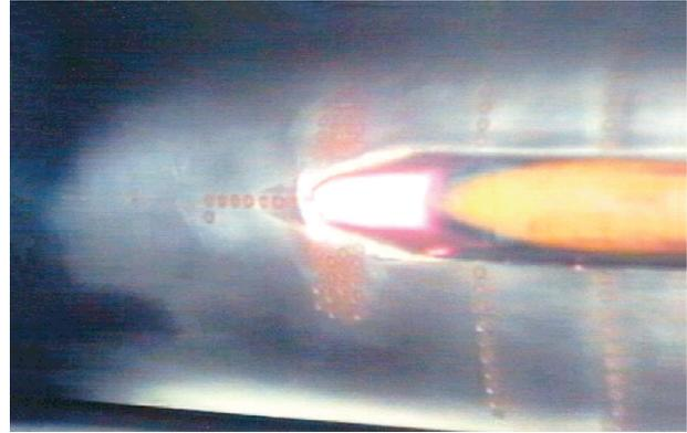
**Figure 13.** Photograph of the strake at maximum heating condition.
