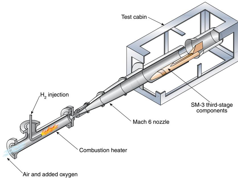
**Figure 11.** Schematic of the AATDL wind tunnel facility. Test setup for SM-3 third-stage insulation materials is shown.
