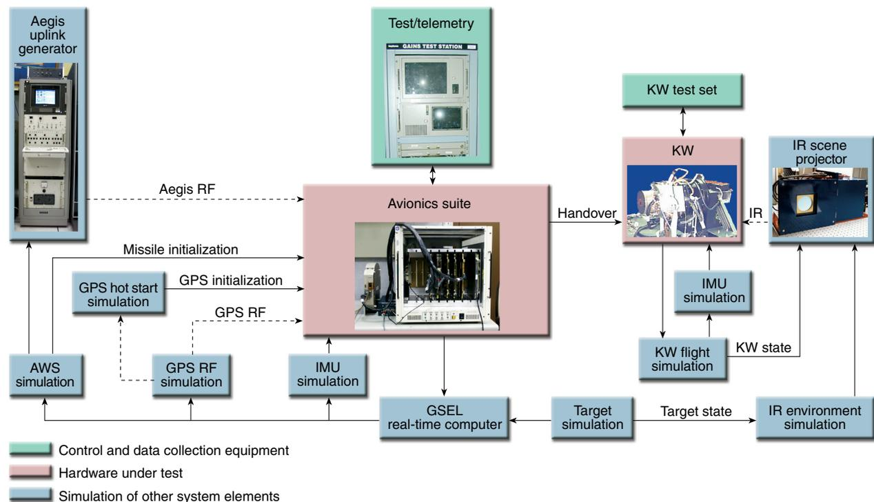
Figure 6. GSEL test configuration.
