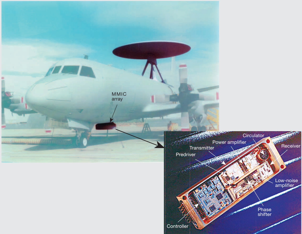
Figure 18. Prototype airborne MMIC array. The photograph shows the CEC cylindrical phased array antenna installed on the U.S. Customs P-3 aircraft. The enlarged area shows one of the prototype MMIC modules used in the array.
