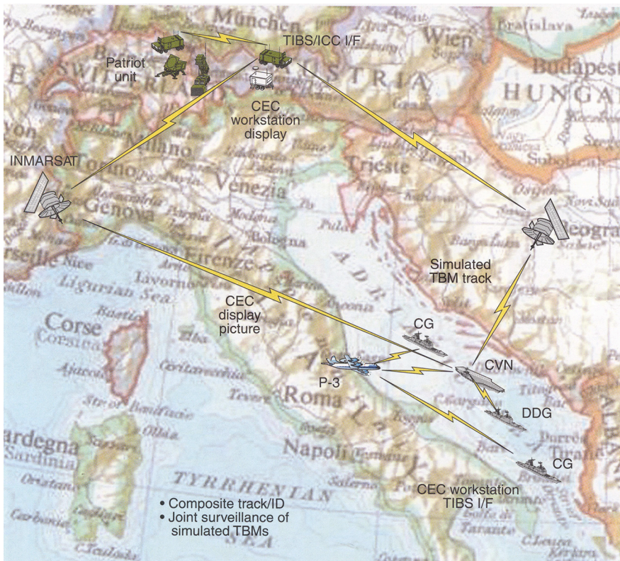
Figure 16. CEC display with part of the battlegroup in the Mediterranean. Shown is the network of the P-3 aircraft, USS Anzio (CG-68), USS Kidd (DDG-993), and USS Dwight D. Eisenhower (CVN-69) with the composite tracks in the Adriatic Sea. (TIBS/ICC I/F = Tactical Information Broadcast System/Integrated Command and Control Interface.)
