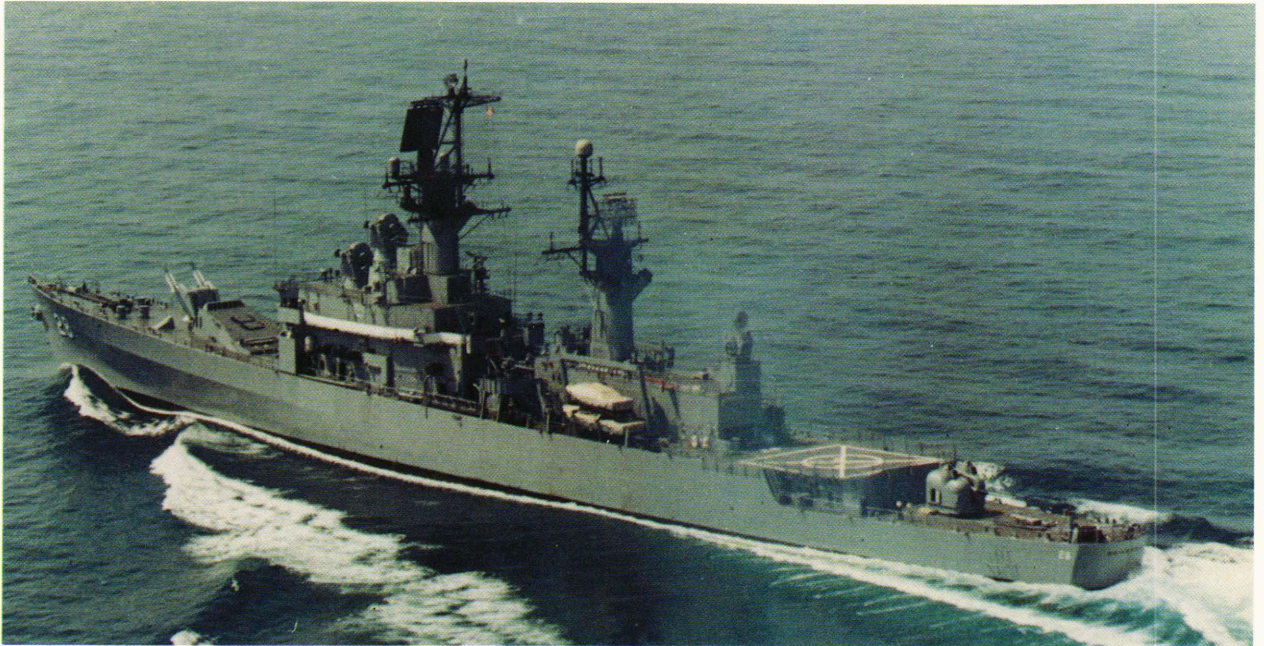
Figure 3 — USS WAINWRIGHT was commissioned in 1966. It was the first all up guided missile frigate, later redesignated as a cruiser, in the combat system configuration that served as the prototype for the TERRIER Modernization Program: AN/SPS-48 Three-Dimensional Air Search Radar, Mk 11 Weapon Direction System, and AN/SPG-55B Fire Control Radars. By 1974, all 31 TERRIER ships were of the modernized configuration.
