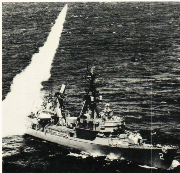
Figure 2 — USS CHARLES F. ADAMS was the first United States guided missile destroyer employing the TARTAR Missile System. USS CHARLES F. ADAMS and USS DEWEY were the first newly constructed ships specifically designed and constructed to be guided missile ships. USS DEWEY was commissioned in 1959 and USS CHARLES F. ADAMS in 1960.
