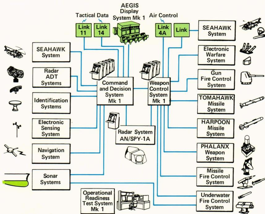
**Figure 2** — The major elements of the AEGIS Combat System perform the basic functions of detection, control, and engagement in anti-air, antisubmarine, and anti-surface warfare.
