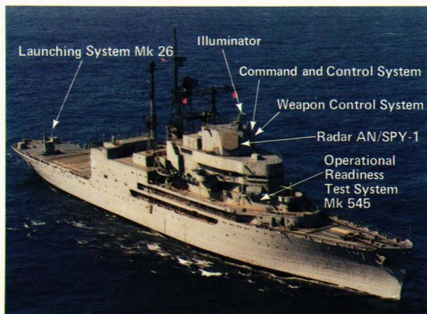
**Figure 6** — AEGIS Engineering Development Model 1 was installed in USS NORTON SOUND, where extensive tests and evaluations of the weapon system have been conducted since 1974.
