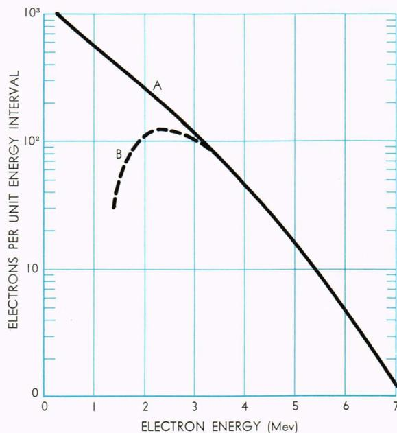
**Fig. 1—(A) Assumed energy spectrum of fission electrons, and (B) energy spectrum of fission electrons counted by the 302 Geiger counter in the TRAAC satellite.**
