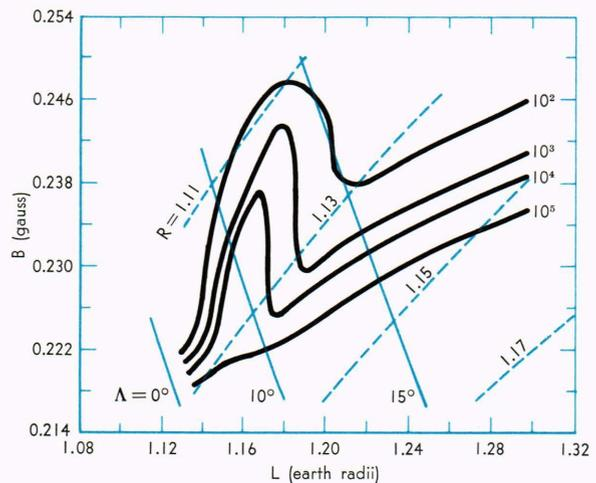
**Fig. 5—Flux contours in  $B$ - $L$  space determined by the TRAAC 302 Geiger counter from Days 192 to 199, longitude region  $\sim 180^\circ\text{E}$  to  $\sim 230^\circ\text{E}$ . Contours refer to omnidirectional flux of electrons of energy  $> 1.6$  Mev in particles/cm<sup>2</sup>-sec. Also shown is a grid in  $R$ - $\Lambda$  space to aid in visualizing the second artificial radiation belt created by the July 9 nuclear burst.**
