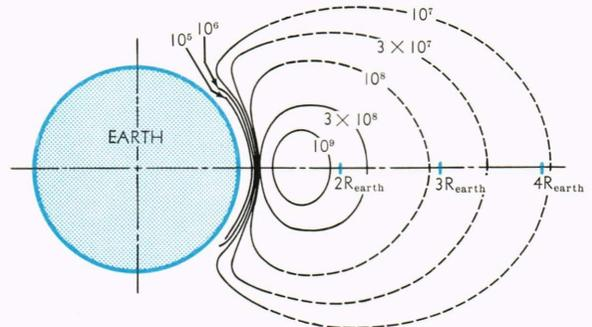
**Fig. 4—Flux contours for the artificial radiation belt in  $R$ - $\Lambda$  space obtained by transformation from Fig. 3.**
