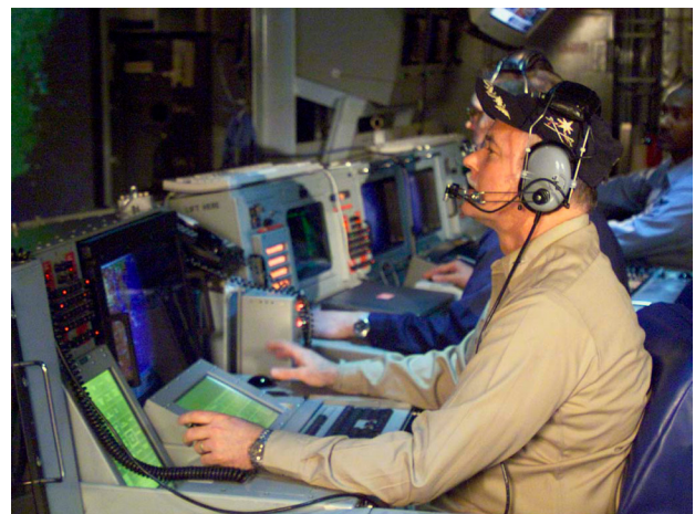
Figure 3. CEC being operated aboard USS Cape St. George . APL conceived and provided technical leadership with collaborating partners in industry and warfare centers on behalf of the sponsor to develop CEC. CEC networks multiple radars to provide fire control-quality composite tracking of aircraft and missiles.
