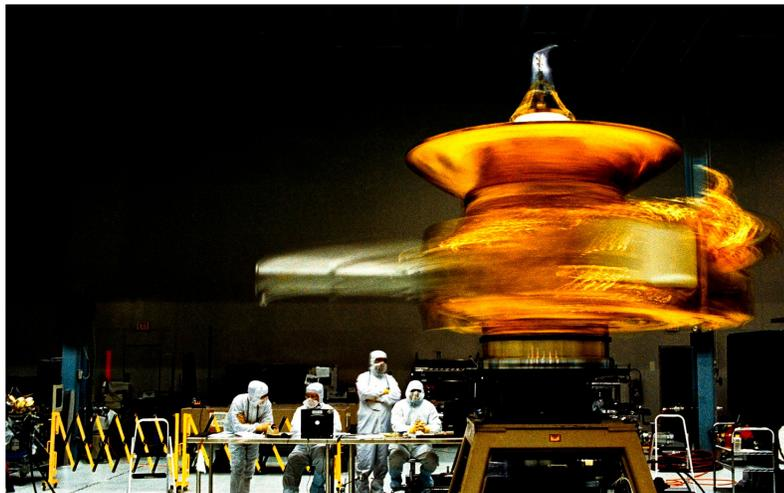
Time-elased photo of the spacecraft spin balance test at NASA Goddard Space Flight Center in June 2005.
