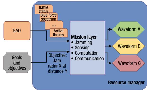
**Figure 6.** Overview of the mission layer and potential outputs. The SAD checks battle status to verify the authority to engage and then selects the jamming waveform among waveform A (most optimal), waveform B (optimal), or waveform C (less optimal),
