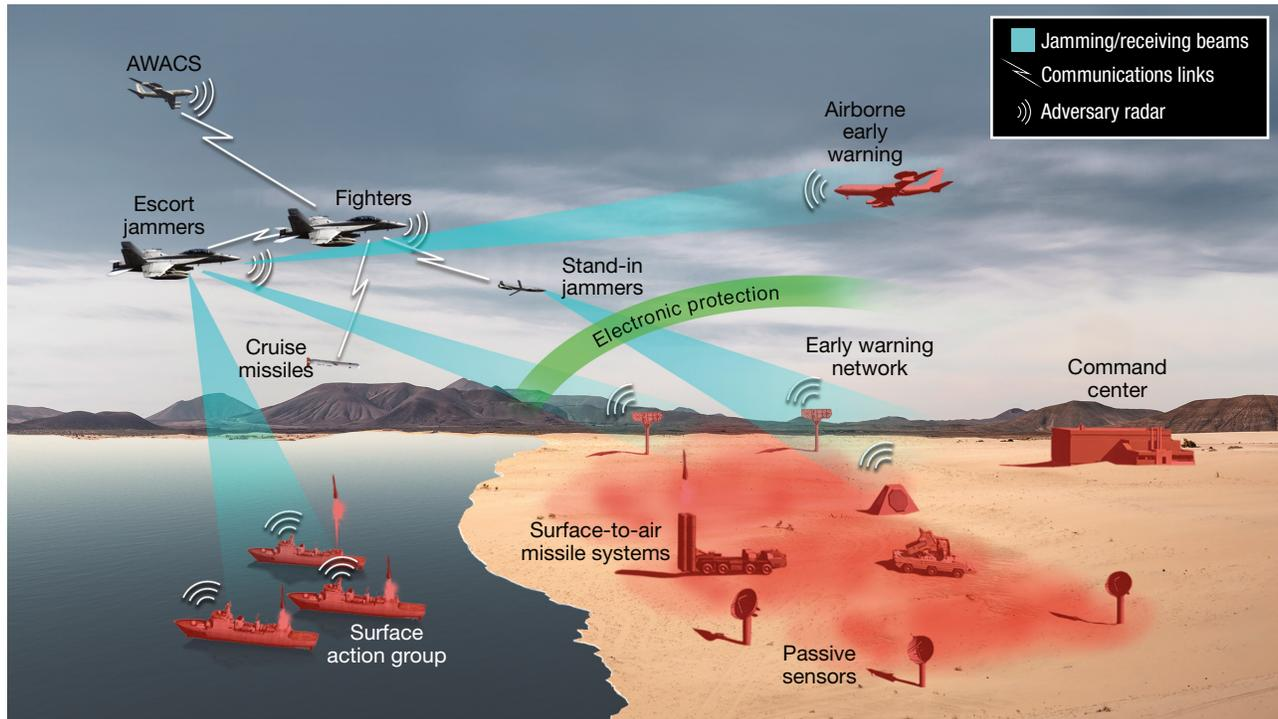
**Figure 1.** An airborne EW network. This diverse network engages naval and ground radar and surface-to-air missile assets. AWACS, airborne warning and control system.
