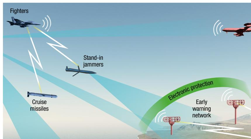
**Figure 5.** Example scenario. In this example, the mission goal is to jam the target early warning network so that the Blue force cruise missiles can reach their objective without being detected by the Red force.
