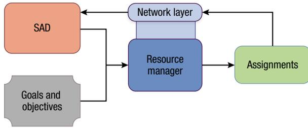
**Figure 3.** Resource management architecture's inputs and outputs. The backbone of the resource management architecture, the network layer moves information to and from nodes and the resource manager and adopts the OSI model to allow for flexible design when creating connections between EW platforms.
