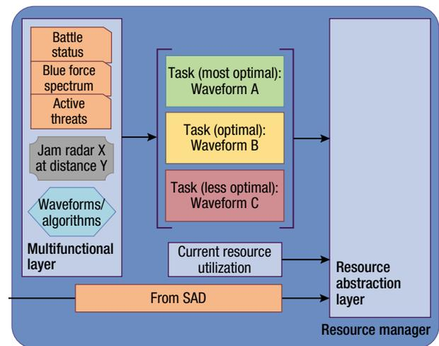
**Figure 9.** The resource abstraction layer taking all provided inputs to provide a final decision to the action layer. The layer configures the action layer to execute waveform A (i.e., configure the sensing, processing, and transmit resources).
