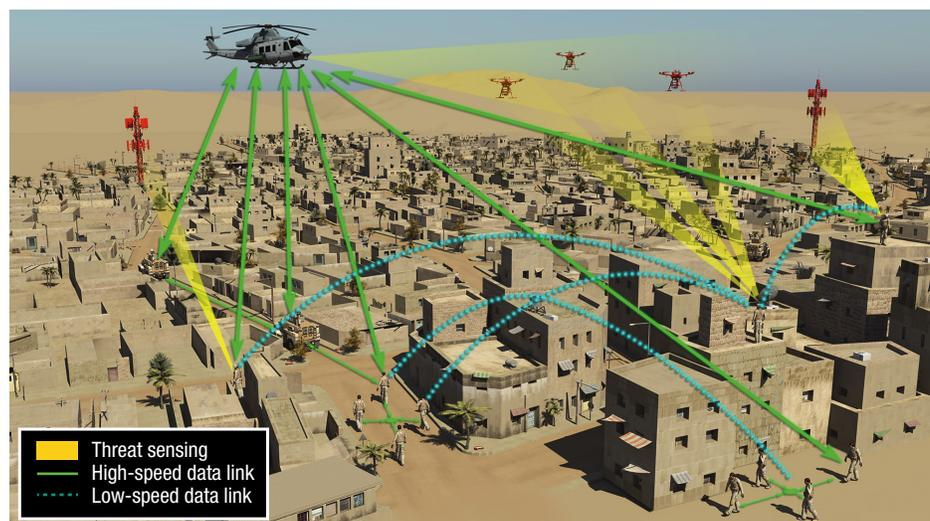
**Figure 2.** A ground EW network. In this scenario, vehicles, body-worn systems, and a helicopter must interact to better engage existing cellular networks and adversary unmanned aerial vehicles.
