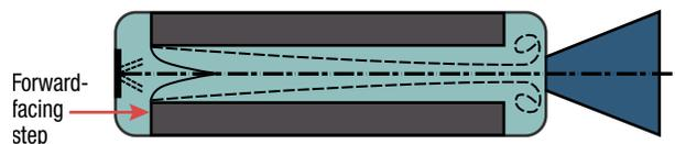
**Figure 8.** Forward-facing step in a hybrid rocket motor. The forward-facing step of the fuel grain promotes favorable gasification of the oxidizer for stable combustion and improved combustion efficiency.
