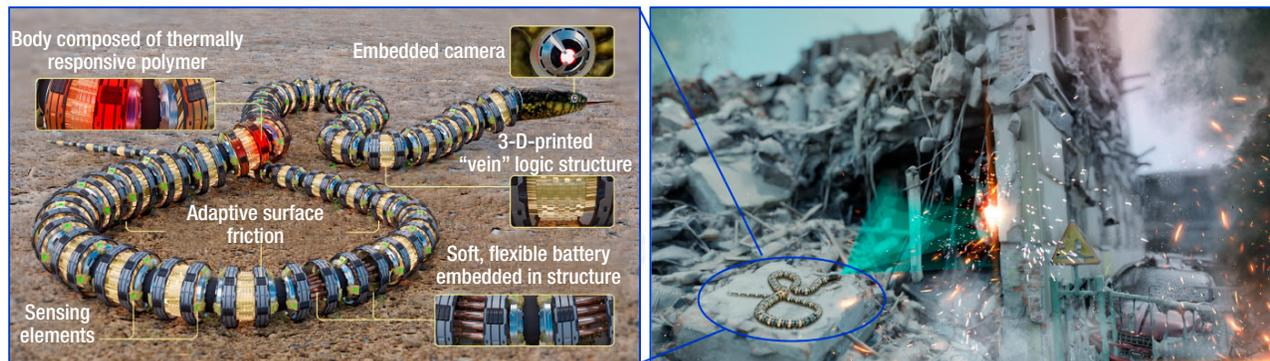
**Figure 4.** The robosnake. The vision for a soft, untethered robosnake integrates a variety of technologies and can be used for both Department of Defense and civilian applications.
