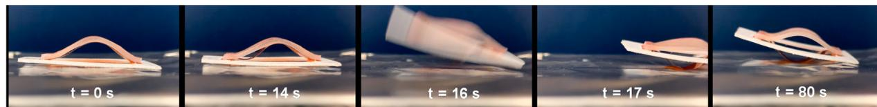
**Figure 3.** A snapping robot using a bilayer LCE/Kapton structure adhered to a polymeric rectangular frame. Activation led to a fast actuation ( $< 2 \text{ s}$ ) resulting in jumping.
