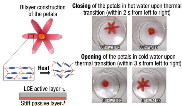
**Figure 1.** Bilayer structures made of LCE and silicone tape for demonstration of bending actuation in a flower shape. Conductive heat transfer to/from liquid enables rapid switching between open and closed state.
