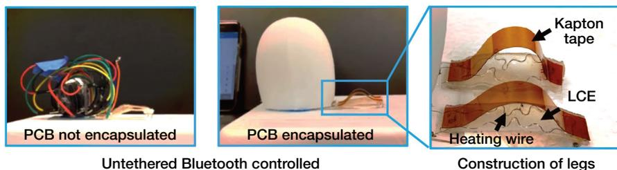
**Figure 2.** Bluetooth-controlled untethered soft robotic systems. Left, Snail robot with the printed circuit board (PCB) not encapsulated. Middle, The same system with the PCB fully encapsulated. Right, a close-up of leg construction. The controlling unit is encapsulated inside the white shell made by 3-D printing.
