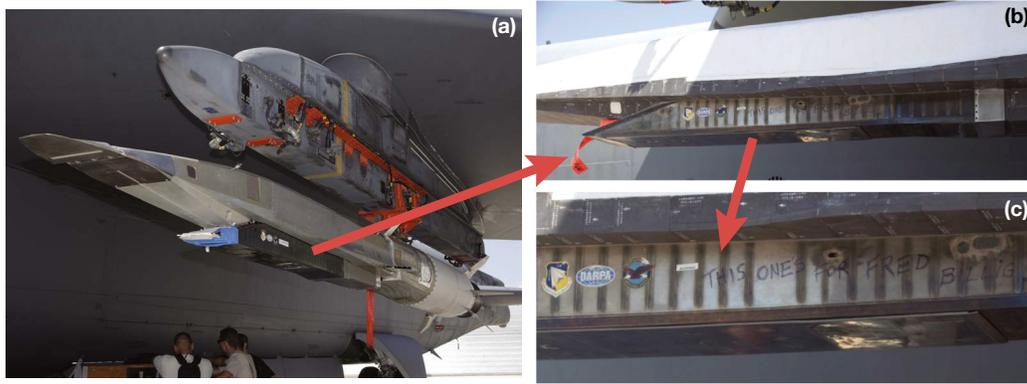
**Figure 3.** X-51A tribute to Dr. Frederick Billig, a pioneer in the development of the scramjet engine. (a) X-51A first flight vehicle mounted on the pylon of the B-52 test aircraft. (b) Close-up view of the hydrocarbon-fuel-cooled metallic scramjet engine. (c) Further close-up view of the scramjet engine with the words “THIS ONE’S FOR FRED BILLIG” written on it. (See acknowledgments for image credits.)
