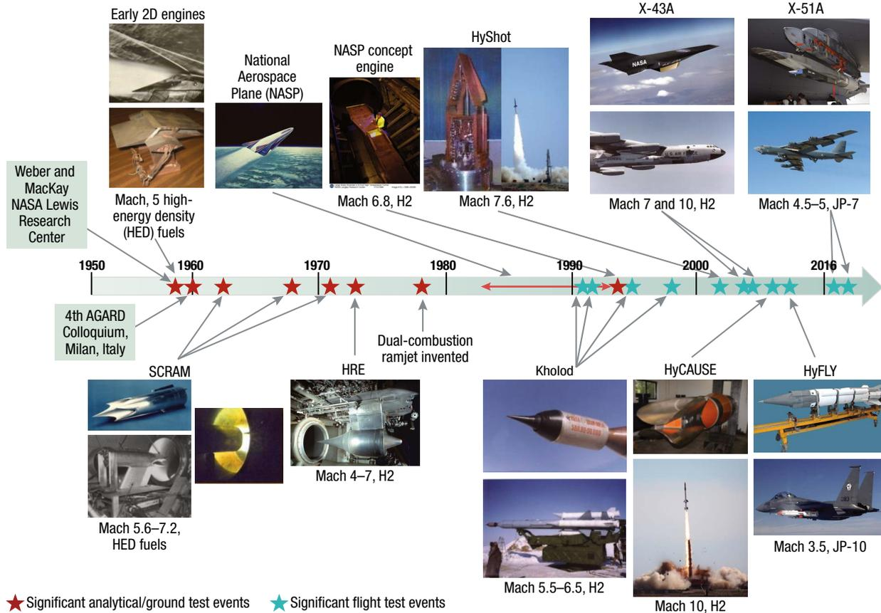
**Figure 2.** Timeline showing major milestones for scramjet development. Red stars indicate significant analytical and ground test milestones. Blue stars indicate significant flight test milestones. The top portion shows the development of planer engine technology. The lower portion shows axisymmetric and 3-D configurations. (See acknowledgments for image credits.)
