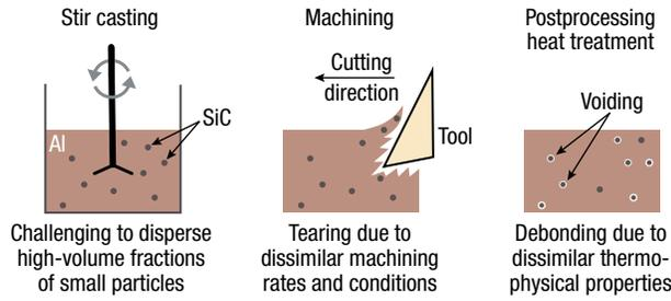
**Figure 1.** Processing challenges in MMCs. Challenges persist across all stages of production: synthesis (e.g., stir casting), machining, and thermomechanical processing (e.g., heat treatments).
