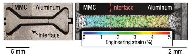
**Figure 6.** A millimeter-scale tension sample. Shown is a dog bone sample across the MMC interface with respective strain in the gauge. The failure occurs in the base metal, indicating that the MMC and interface are not the weak link in the system.
