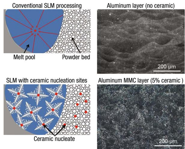
**Figure 4.** A dark-field microscopy comparison of the microstructure of a conventional SLM material compared to an MMC material. The unique melt pool structure to SLM can be seen in the non-ceramic material where it is absent in the MMC.
