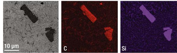
**Figure 3.** Images showing that APL's SLM system was able to produce Al-SiC MMCs. A scanning electron microscopy image and the corresponding elemental maps from energy-dispersive x-ray spectroscopy of the solidified Al-SiC MMC formed via SLM.
