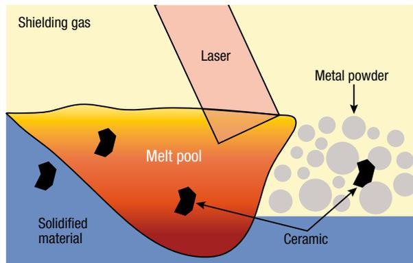
**Figure 2.** Graphical depiction of a hybrid metal–ceramic powder mixture used in SLM. This blended powder bed can be used to generate a ceramic-reinforced material with minimal modification to the SLM process.
