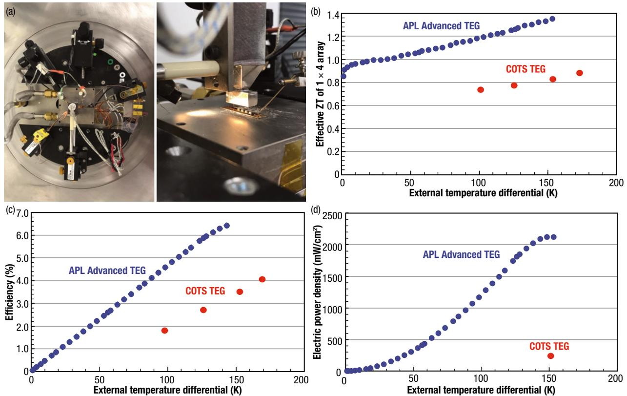
**Figure 2.** Setup and results. Experimental setup for testing thin-film thermoelectric devices (a) and performance curves that describe the advancements achieved over commercial off-the-shelf (COTS) thermoelectric devices, including (b) effective ZT as a function of temperature, (c) thermal-to-electric conversion efficiency, (d) and electric power density.
