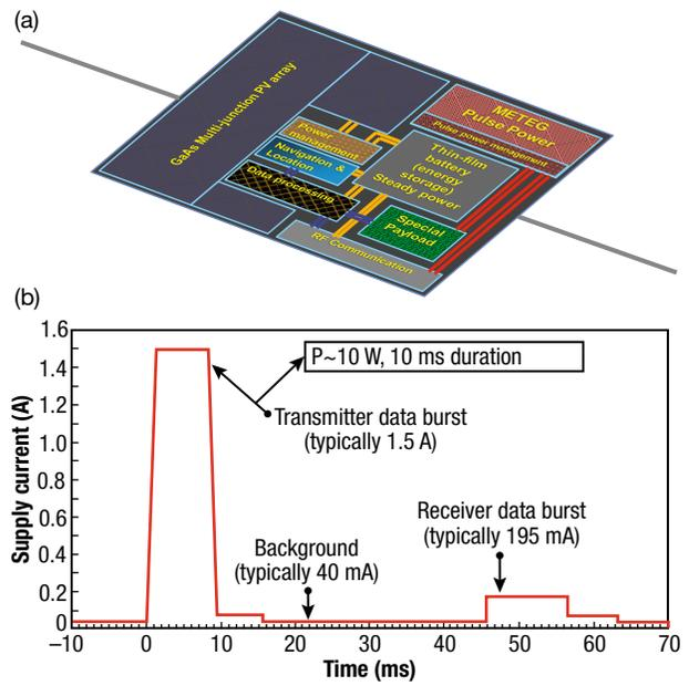
**Figure 1.** Microscale energetic thermoelectric generators (METEG) applications. (a) New-generation small-scale satellite systems like chip-scale satellite systems<sup>1</sup> and (b) RF communication devices in ground systems can benefit from METEG pulse power sources.
