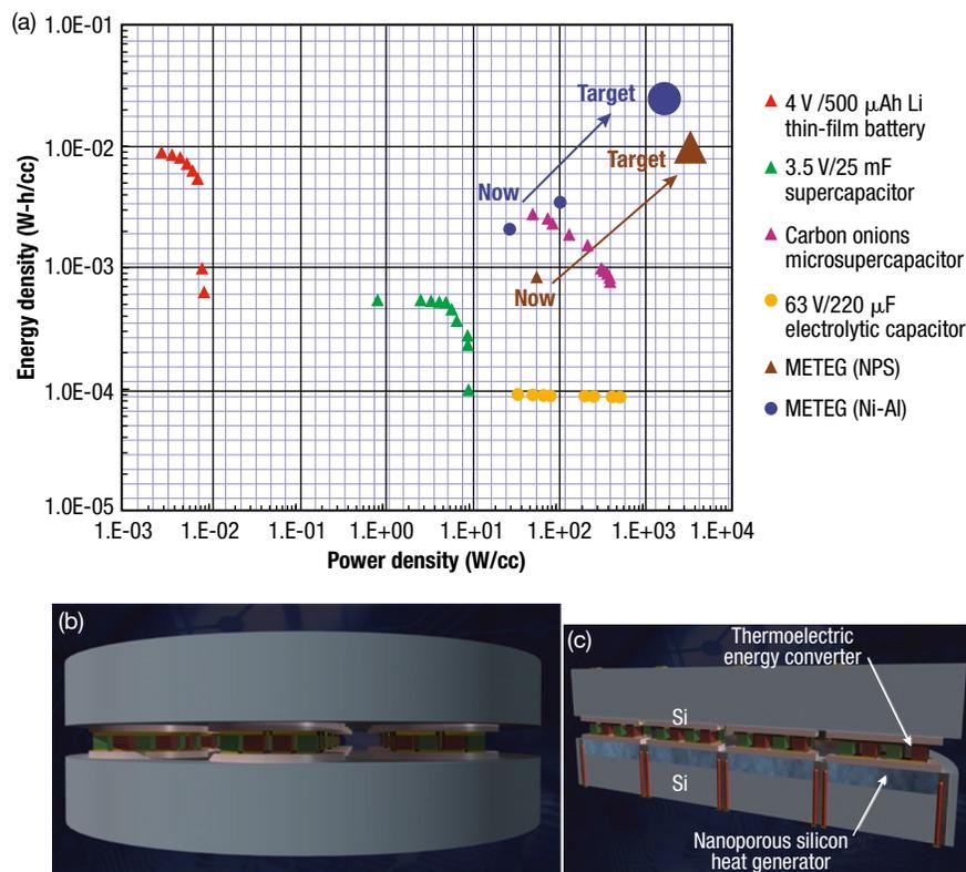
**Figure 3.** Capabilities and details of the METEG concept. Top, Plot of energy density versus power density for a variety of technologies such as lithium-ion batteries, electrolytic capacitors, supercapacitors,<sup>5</sup> and METEG technologies developed in this effort; bottom left, schematic of a compact, packaged METEG device that can be developed based on the reported results; bottom right, inner details of the METEG device showing the thermoelectric converter and other aspects.
