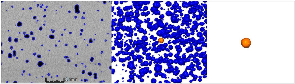
**Figure 2.** XRCT data processing techniques for identification of porosity in an AlSi<sub>10</sub>Mg AM specimen. The defect structure is seen in the 2-D slice (left) and can be segmented in 3-D (middle) and uniquely quantified (right).
