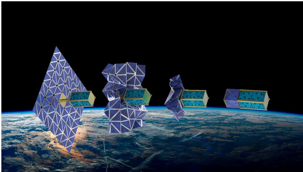
**Figure 3.** Vision of APL study. Combining the functional properties of shape memory alloys with 3-D printing to develop next-generation deployable space structures.
