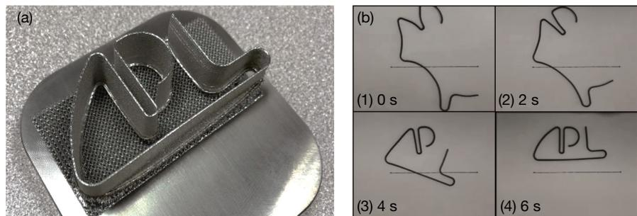
**Figure 2.** Proof-of-concept demonstration. This figure shows that our optimized processing parameters and lattice support approach successfully translates to complex, large-scale, shape-memory components. (a) APL logo part ( $65 \text{ mm} \times 32 \text{ mm} \times 20 \text{ mm}$ ) built on a lattice. (b) Time stamps of deformed logo undergoing shape recovery upon heat exposure. (Reprinted with permission from Ref. 10.)
