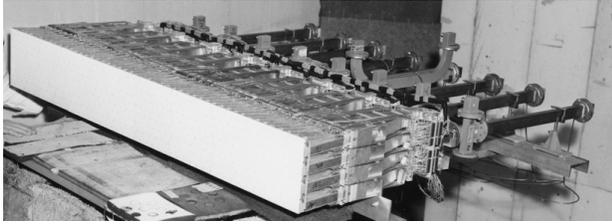
**Figure 1.** Photo of the front of the AMFAR phased-array antenna. AMFAR was the prototype for the Aegis SPY-1 radar.
