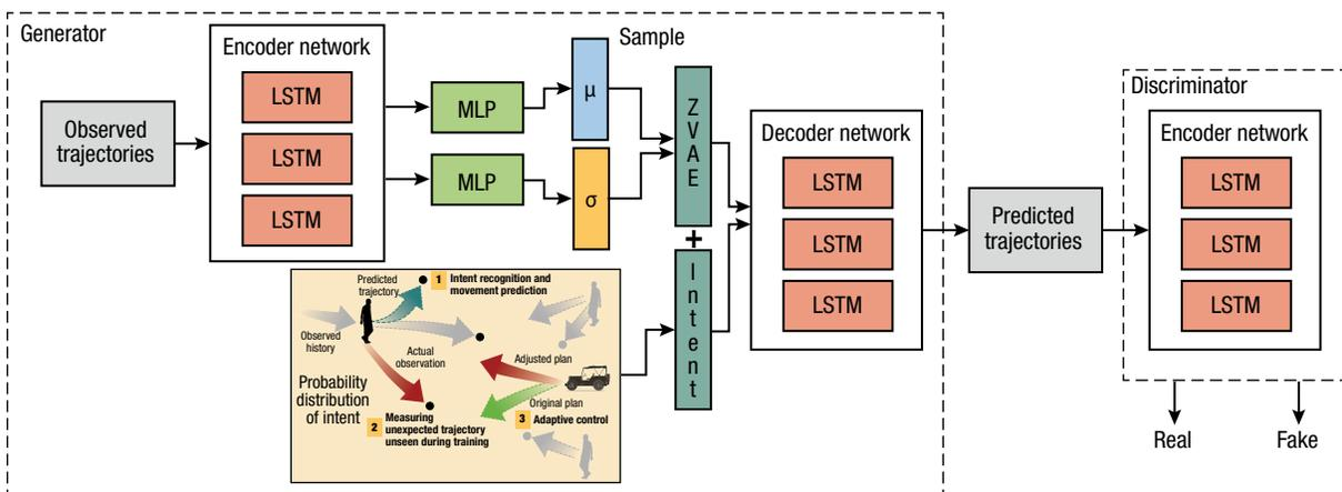
**Figure 2.** Pedestrian prediction neural network architecture. We first estimate a probability distribution of the intent of the pedestrian and then combine that estimation with past trajectories using long short-term memory (LSTM) and multilayer perceptron (MLP) neural networks. The network learns a Gaussian representation that can be sampled from and combined with the intent to predict future pedestrian motion. © 2020 IEEE. Modified and reprinted, with permission, from Ref. 1.)
