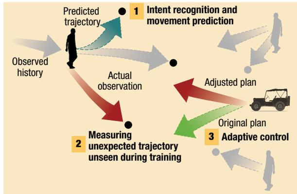
**Figure 1.** Our approach for adaptive crowd navigation. (1) We first estimate the intent of the pedestrian and combine the estimation with past trajectories to predict future motion. (2) We then measure the error between our prediction and reality to develop an adaptive mobile robot controller. (3) The adaptive mobile robot controller switches between aggressive and risk-averse policies based on accuracy of the prediction. © 2020 IEEE. Modified and reprinted, with permission, from Ref. 1.)
