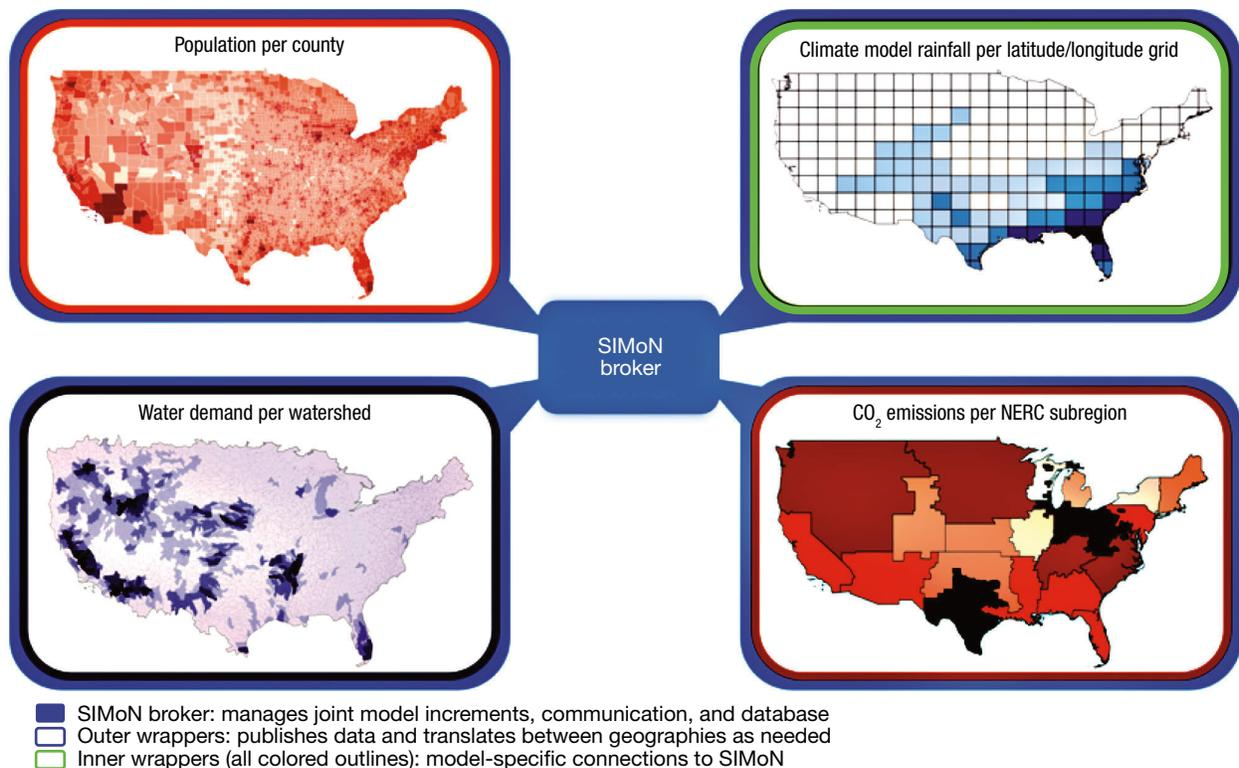
**Figure 1.** SIMoN architecture diagram with model output snapshots from the year 2050. Note: These results are intended to demonstrate SIMoN modeling communication and should not be taken at face value until model validation efforts are completed. (© 2020 IEEE. Adapted, with permission, from Hughes et al.<sup>1</sup>)
