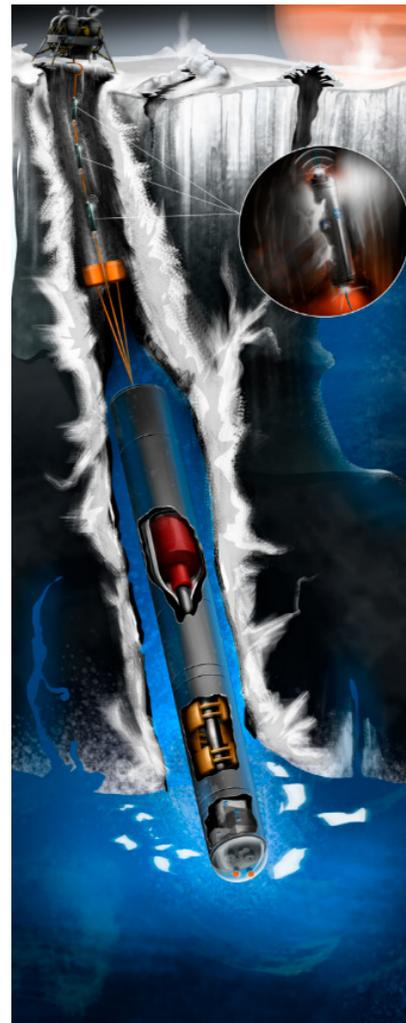
**Figure 10.** Artist’s concept of a cryobot traversing the ice shell and reaching the ocean. (NASA image from Oleson et al.<sup>54</sup>).
