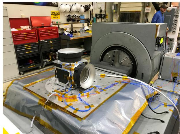
**Figure 7.** Europa Clipper PIMS engineering model set up for microphonics and vibration testing. PIMS, being developed at APL, is a Faraday cup-based plasma spectrometer. Its measurements will help fully constrain Europa's ocean depth and salinity, as well as its ice shell thickness.
