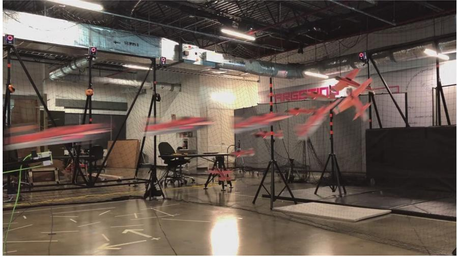
**Figure 2.** Time-lapse image showing a small fixed-wing aircraft performing a sharp 90° turn. Two striped poles denote the goal point for the maneuver.<sup>5</sup>
