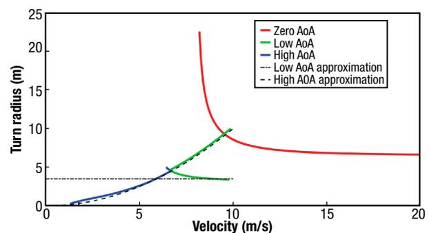
**Figure 1.** Demonstration of how fixed-wing UAVs achieve smaller turn radii by executing high-AoA maneuvers. Curves were generated by computing turn trim conditions using a nonlinear program and a simplified nonlinear aircraft model without control surfaces. Constraints were placed on the AoA to demonstrate the advantage of post-stall turns.<sup>5</sup>
