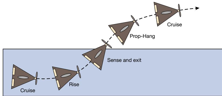
**Figure 4.** Diagram of flight behavior during a water-exit maneuver. Real-time state estimation is used to detect the transition point as the vehicle exits the water.
