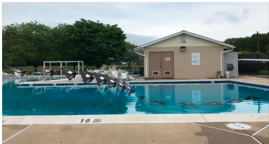
**Figure 5.** Time-lapse image of a successful water-exit maneuver. The Flying Fish approach, combined with onboard state estimation to detect transitions between dynamics regimes, enables the vehicle to autonomously exit a body of water and enter forward flight.
