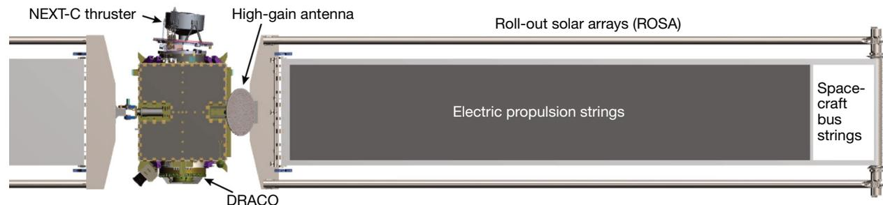
**Figure 7.** DART's mechanical layout. The layout is dominated by accommodation of the NEXT-C thruster and ROSA. DRACO, Didymos Reconnaissance and Asteroid Camera for OpNav.
