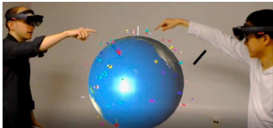
Figure 4. ARMOUR X collaborative experience. Two users, each wearing a Microsoft HoloLens and using an Xbox controller, interact with the system simultaneously.
