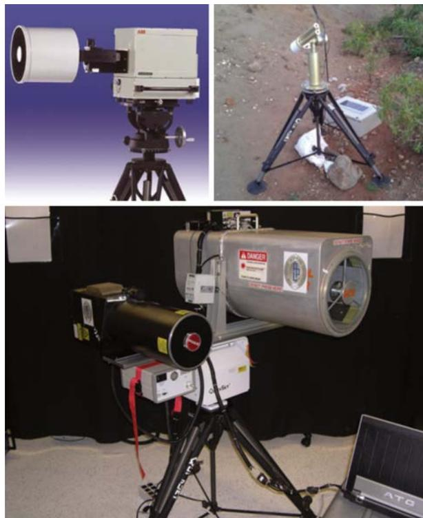
**Figure 28.** Images of the FTIR (upper left), micropulsed lidars (lower), and sun photometer systems (upper right) used for atmospheric characterization.
