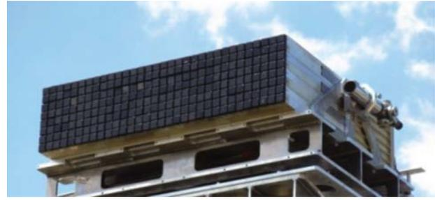
Figure 3. AUSPAR element-level digital array under test.
