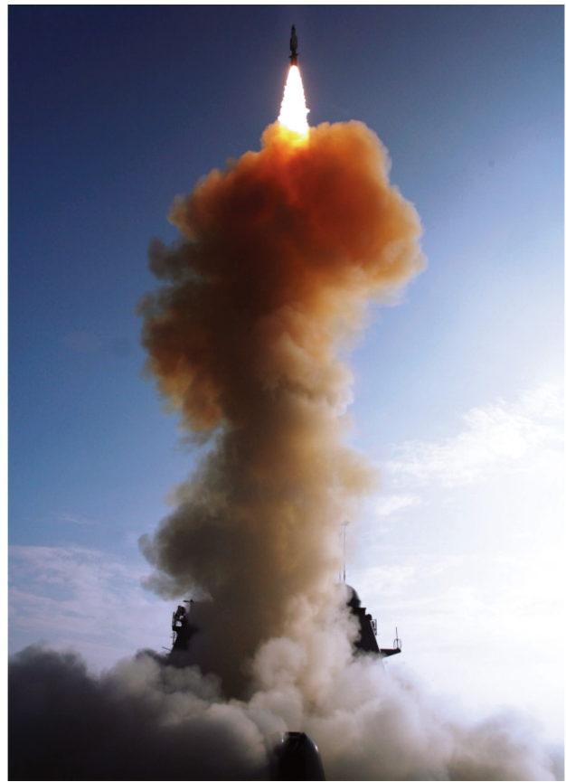
Figure 3. Aegis/SM-3 launch during the Burnt Frost event. This critical operation required the APL, government, and industry team to make rapid modifications to the Aegis BMD System so that it could successfully intercept an errant intelligence satellite and rupture its fuel tank before the satellite reentered Earth's atmosphere.
