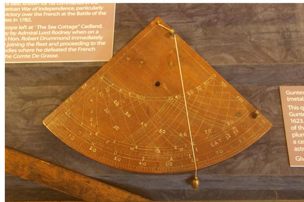
**Figure 2.** Gunter's quadrant, a simplified version of an astrolabe, precursor to the sextant. (Photograph by Mike Peel, www.mikepeel.net; CC BY-SA 4.0, <https://creativecommons.org/licenses/by-sa/4.0>.)
