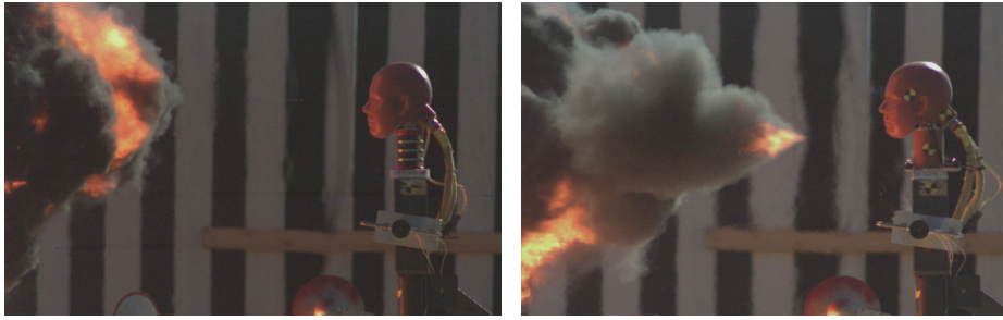
Figure 7. Live-fire blast tests are prone to environmental and experimental artifacts. The image on the left depicts an ideal test in which the headform is subjected to a symmetrical shock wave, and the image on the right depicts debris jetting directly at the headform, despite nominally similar test conditions.
