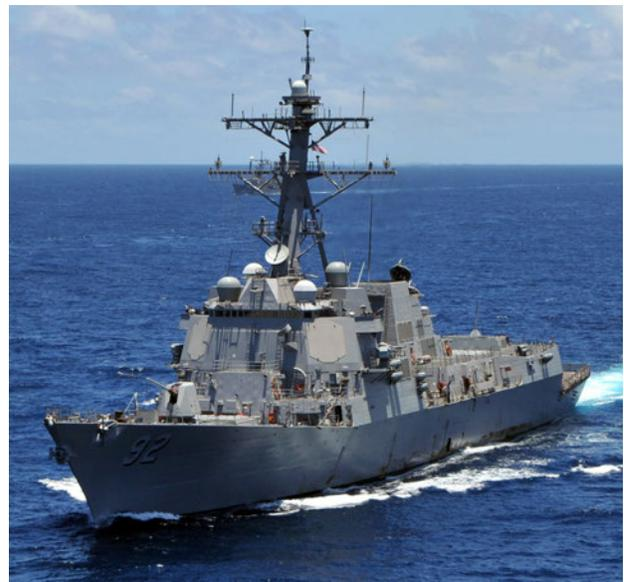
**Figure 3.** USS *Momsen* (DDG 92) with the two AN/SPY-1D(V) radar forward faces visible on the deckhouse. (U.S. Navy photo by Mass Communication Specialist 2nd Class James R. Evans/Released.)
