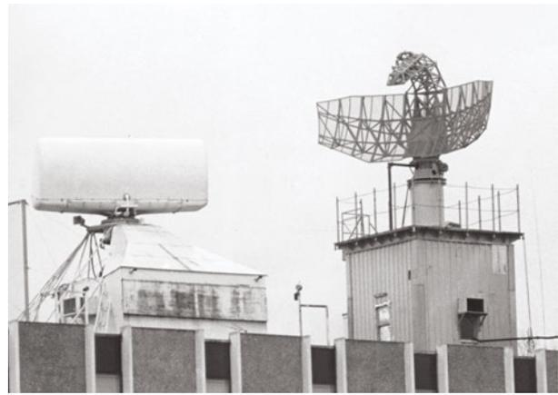
**Figure 1.** APL-developed AMFAR (left) shown in contrast to the conventional rotating reflector radar antenna of the era (right).
