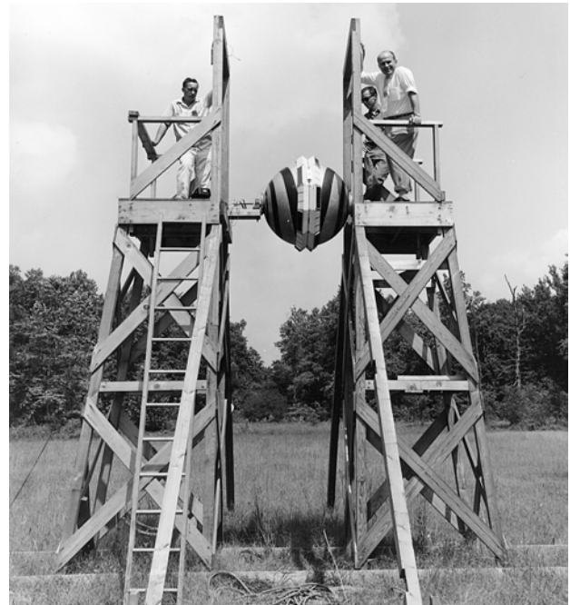
Figure 3. The yo-yo-like de-spinning mechanism being tested on APL's first satellite in 1959, under the philosophy of "test what you fly, fly what you test." James Smola (far right) is conducting the test. Also pictured are Wilfred Zimmerman (left) and David Moss (next to Smola).
