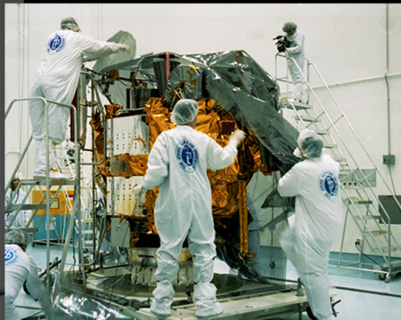
MESSENGER engineers, technicians, and quality assurance in one of APL’s cleanrooms, wrapping the spacecraft for transport. The copper-shaded material on the outside of the spacecraft is a blanket of multilayer insulation, a thermal insulator.
