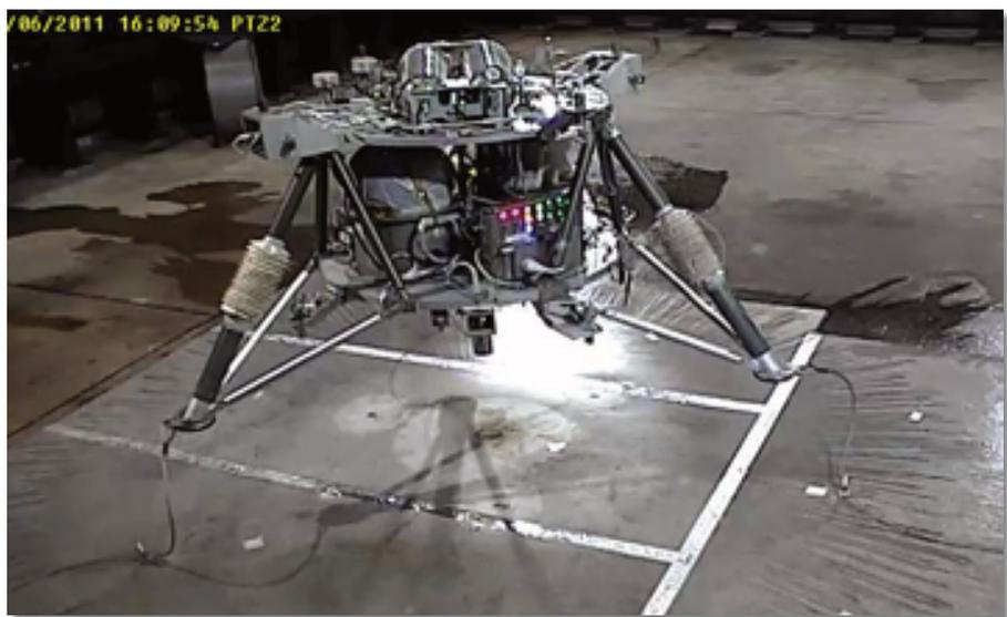
**Figure 9. Tethered indoor flight test. (NASA)**
