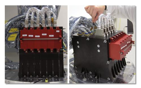
Figure 1. Flight PDU box with nonflight fuse modules.
