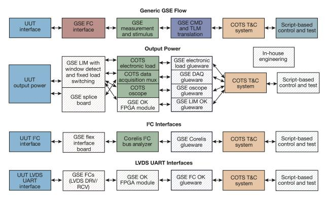
**Figure 3.** Use of COTS equipment within the GSE test flow to reduce in-house engineering complexity. CMD, command; DAQ, data acquisition; DRV/RCV, driver/receiver; FC, first circuit; LIM, load interface module; OK, Opal Kelly; TLM, telemetry; UUT, unit under test.
