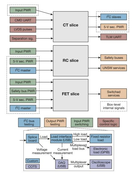
Figure 5. PDU major test interfaces. GPIB, General Purpose Interface Bus; sig., signal; sec., secondary; UNSW, unswitched.
