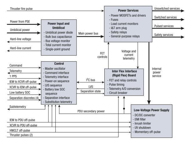
**Figure 2.** RBSP power subsystem block diagram. 1 PPS, 1 pulse per second; EMI, electromagnetic interference; HWCLT, hardware command-loss timer; IEM, integrated electronics module; LVS, low voltage sense; PSE, power system electronics; SOC, state of charge; XCVR, transceiver.
