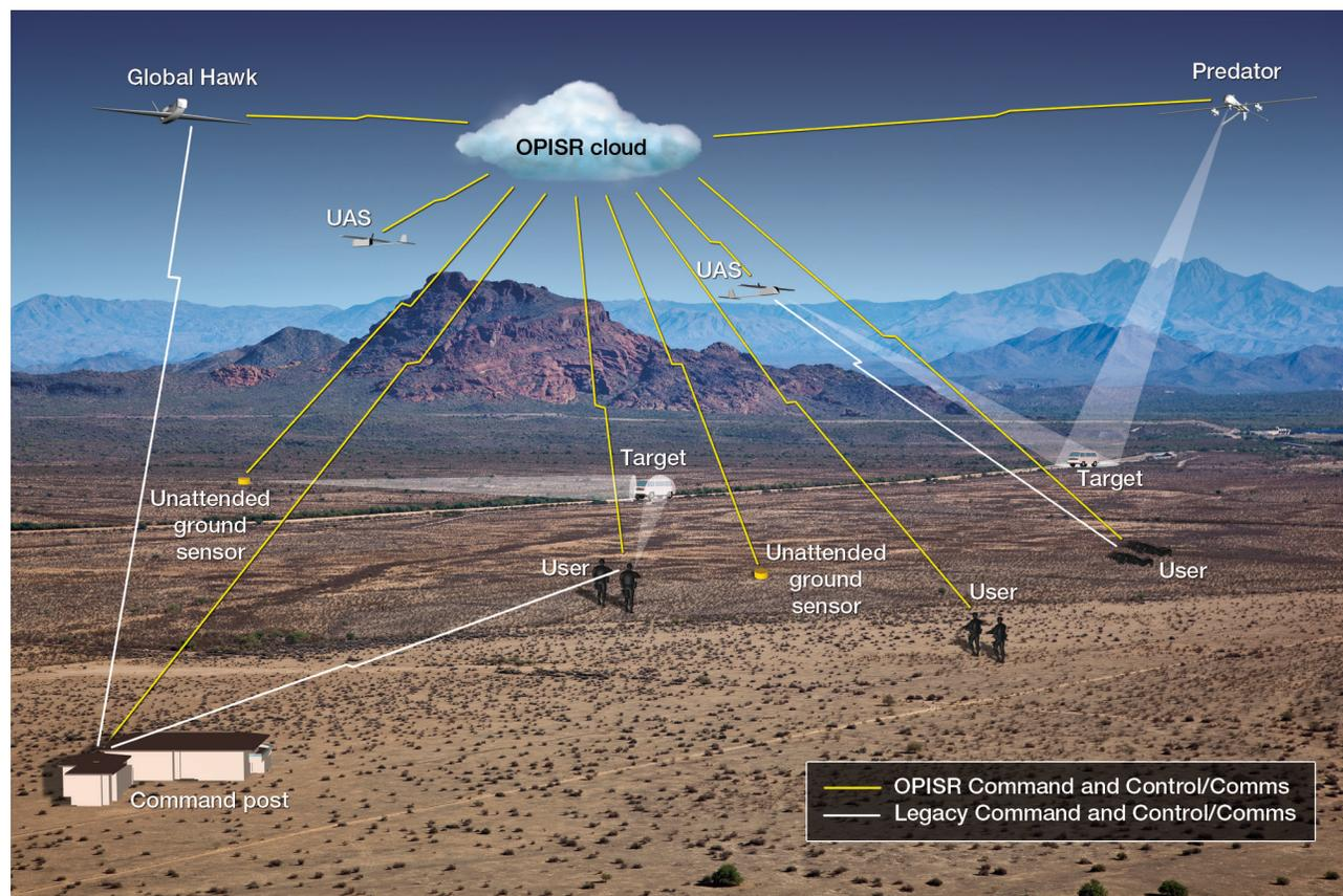
**Figure 2.** OPISR’s concept of operation allows UAVs of various sizes to communicate with each other, with users, and with commanders through an ad hoc, asynchronous cloud. The cloud communicates goals from users to vehicles and sensor observations from users to vehicles. Comms, communications.
