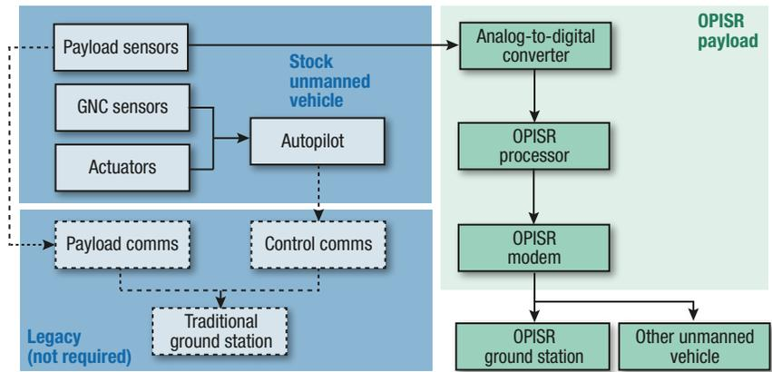
**Figure 3.** OPISR's hardware architecture is based on a modular payload that can be fitted onto different types of unmanned vehicles.
