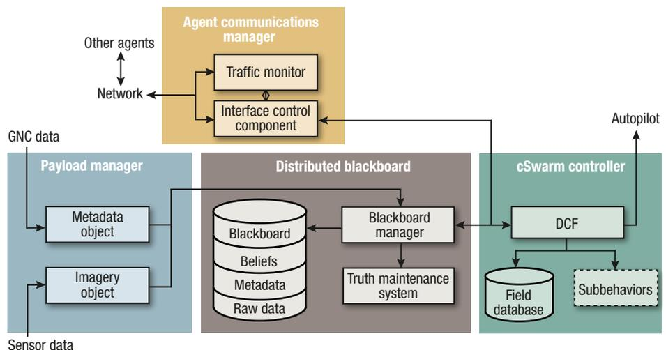
**Figure 4.** OPISR software architecture contains four major elements: the payload manager generates new "beliefs" from sensor observations, the distributed blackboard maintains situational awareness by aggregating beliefs from the on- and offboard observations, the agent communications manager exchanges beliefs between other vehicles and users, and the cSwarm controller devises a course of action based on beliefs. DCF, Dynamic co-fields.
