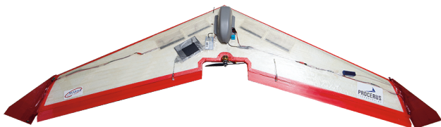
Figure 1. The Procerus Unicorn, which typically has a 5-ft (1.5-m) wingspan.
