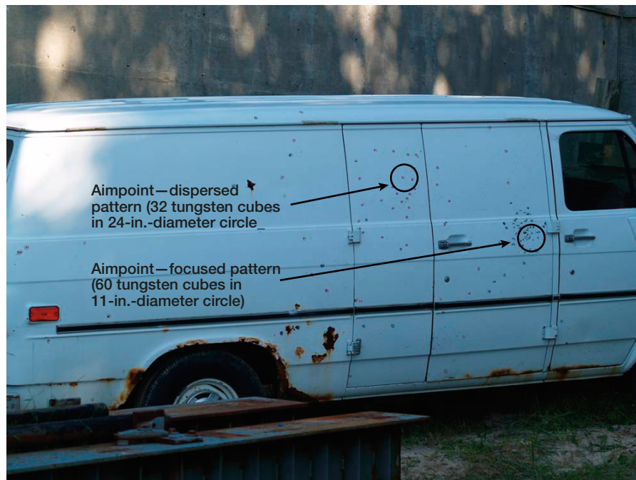
Figure 21. Warhead lethality test results.
