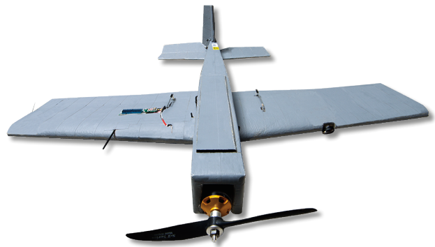
Figure 2. The Procerus Miracle, which has a 3-ft (0.9-m) wingspan.
