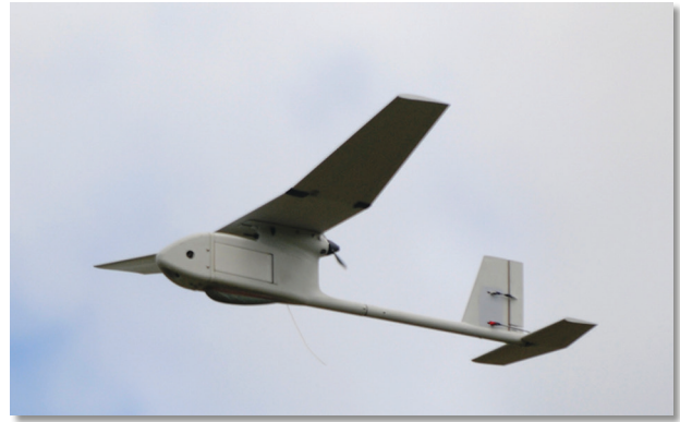
Figure 4. The AeroVironment RQ-11B Raven, which has a 4.5-ft (1.37-m) wingspan. (U.S. Army photo: Staff Sergeant Don Veitch.)
