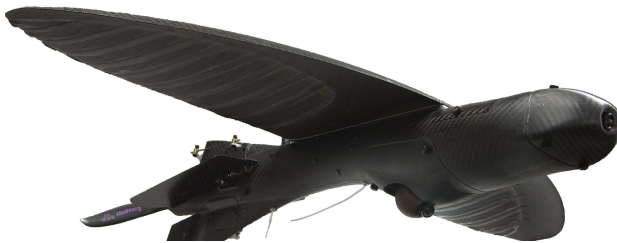
Figure 3. Three views of the Prioria Maveric, which has a 2.46-ft (0.75-m) wingspan. (© 2012 Prioria Robotics.)
