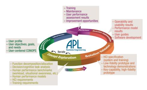
**Figure 10.** Cognitive engineering products within systems engineering. CONOPS, concept of operations; HCl, human-computer interaction.
