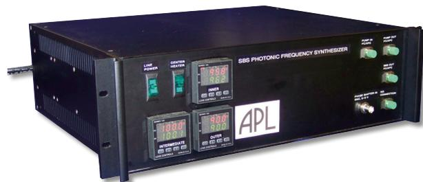
**Figure 4.** Photograph of the rack-mountable chassis containing the SBS laser.
