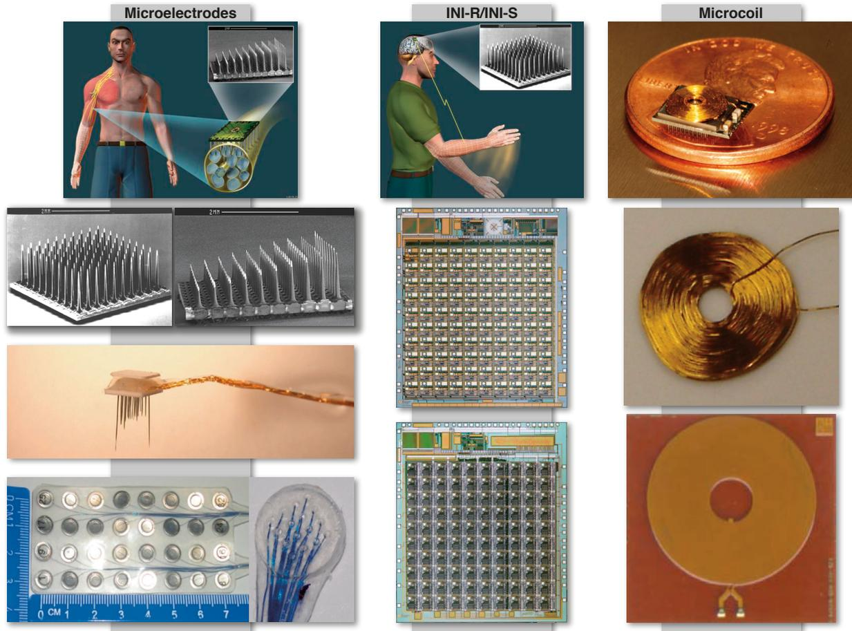
**Figure 14.** Neural interfaces ranged from electrode arrays containing up to 100 arrays within a 16-mm<sup>2</sup> area to custom application-specific integrated circuits and custom-designed coils for wireless power and data transmission. INI-R/INI-S, implantable neural interface recording/implantable neural interface stimulation.
