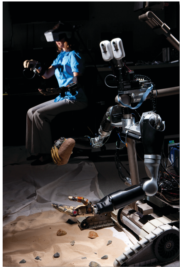
Figure 12. Remote teleoperations enables robotic replication of user movements.
