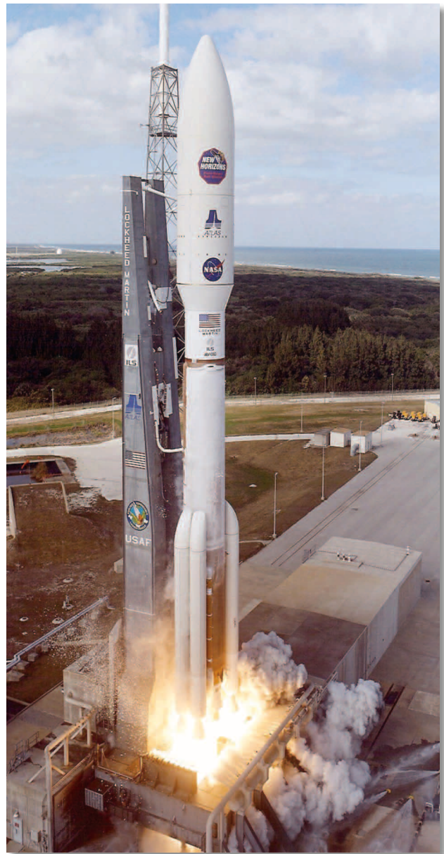
Figure 4. The New Horizons mission, whose design required careful management of spacecraft mass and the largest available launch vehicle (the Atlas V 551).
