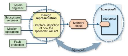
Figure 4. Engine-based design with generic interpreter and data set (memory object).
