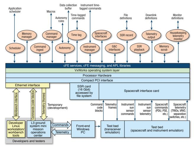
Figure 5. RBSP modular-component software bus architecture. cFe, NASA Goddard's Core Flight Executive; PDU, power distribution unit; PSE, power system electronics; SSR, solid-state recorder; TRIOs, temperature remote input output; VRIO, voltage remote input output.
