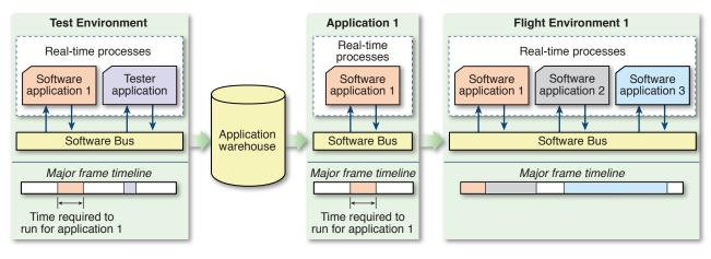
Figure 3. Testing and integration environment.
