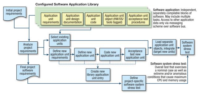
Figure 1. Modular-component development process. CPU, central processing unit; HW, hardware; OS, operating system.
