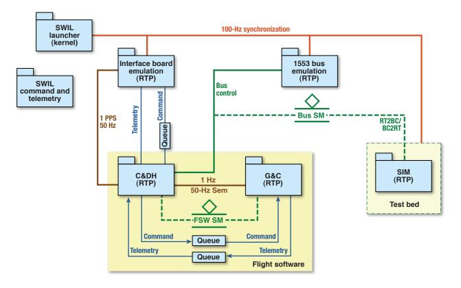
**Figure 6.** SWIL testing where command and data handling (C&DH) software and guidance and control (G&C) software can be tested against hardware emulations and physics-based simulations all within the flight processor. FSW, flight software; PPS, pulse per second; RTP, real-time process; Sem, semaphore; SIM, simulation (dynamics, environment); SM, shared memory.
