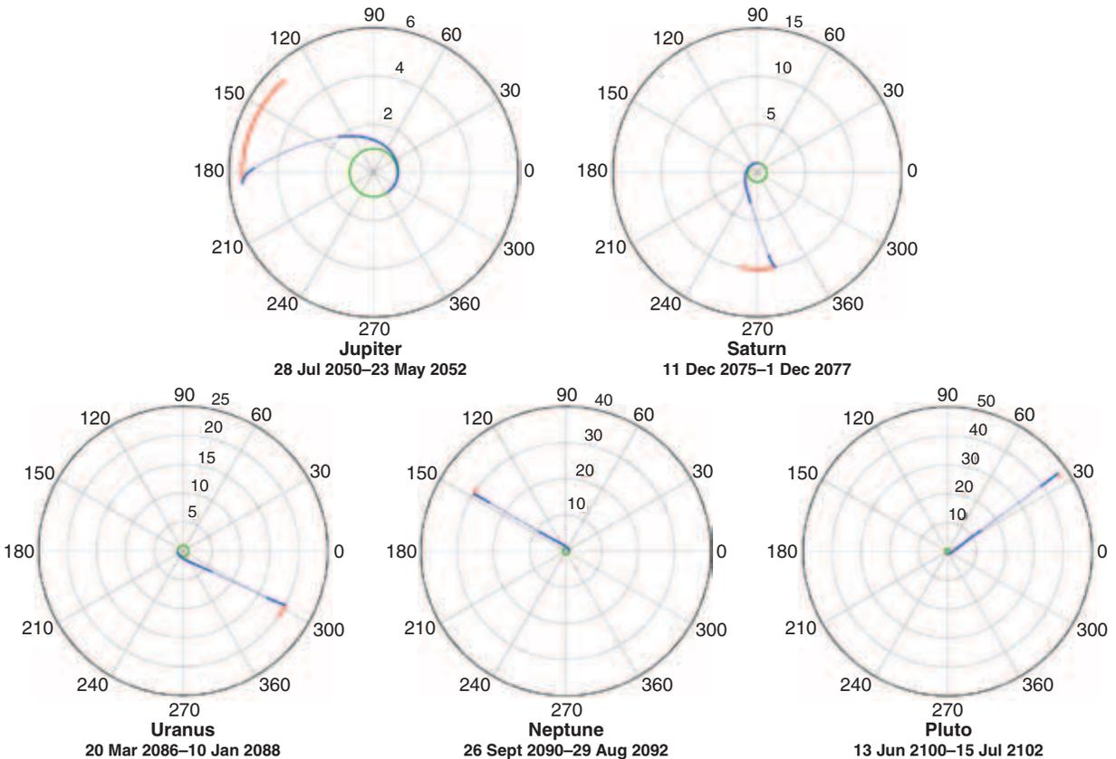
**Figure 3.** Outbound trajectories corresponding to the details of Fig. 2. Projections are into the plane of the ecliptic where 0° is the first point of Aries. Note the different radial scales and increasingly linear trajectories with larger heliocentric distance to the target.
