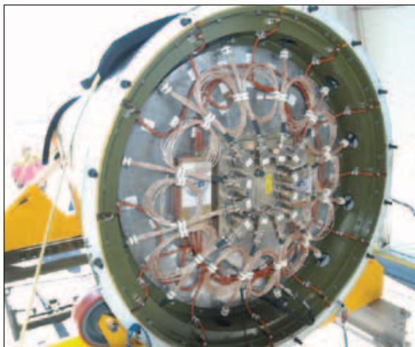
Figure 9. The 12-channel BID is shown installed on the USFT-1 target. The BID comprises the two 6-channel electro-optical modules and 12 high-temperature fiber-optic light guides seen in red. The unit in the center is part of the hit-detector system, which was not provided by APL.
