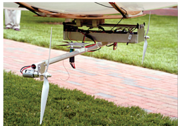
Figure 4. LAURA gondola and motor-propellers provide three-axis position and three-axis attitude control.
