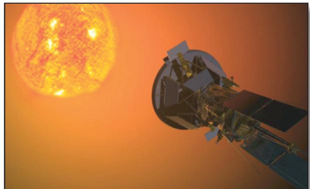
**Figure 1.** The harsh environment of the Solar Probe Plus spacecraft, with solar fluxes 50 times larger than any previous spacecraft has experienced. Newly developed ceramic coatings for the Thermal Protection System will help protect the spacecraft in this harsh environment.
