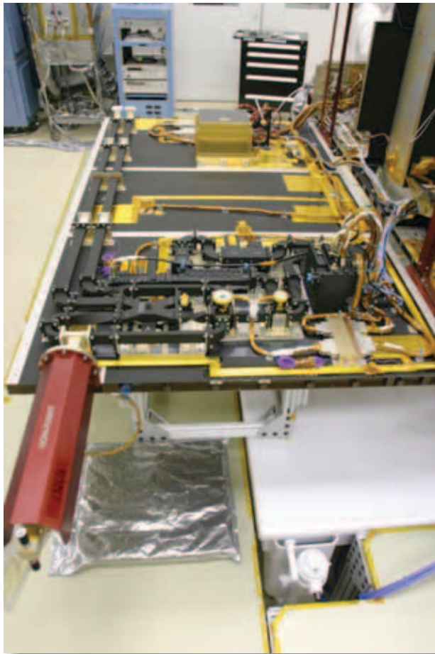
Figure 10. STEREO -y deck before flight closing. Note the extensive run of X-band waveguide across the deck.
