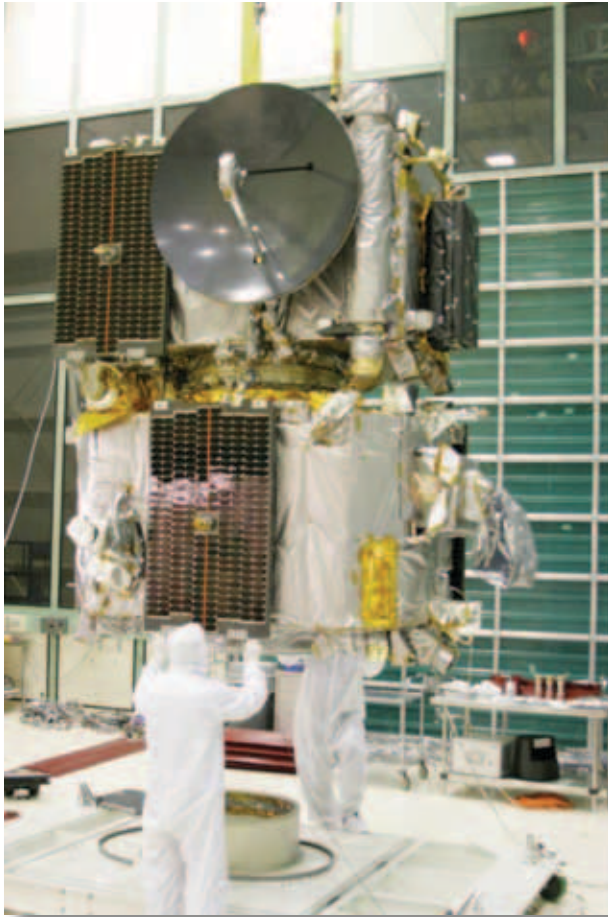
Figure 8. Lifting operation of STEREO flight stack.
