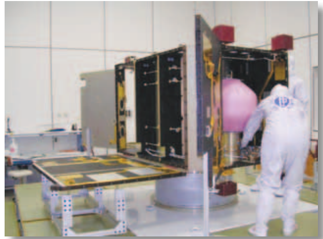
Figure 9. STEREO A, after propulsion system integration, with all decks opened.
