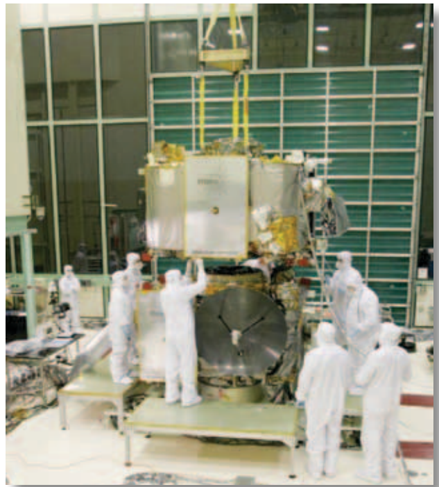
Figure 7. Stacking operation of STEREO A onto STEREO B.
