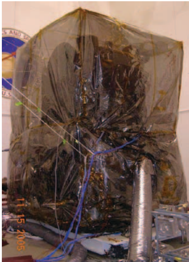
Figure 22. STEREO observatory stack acoustic test configuration.
