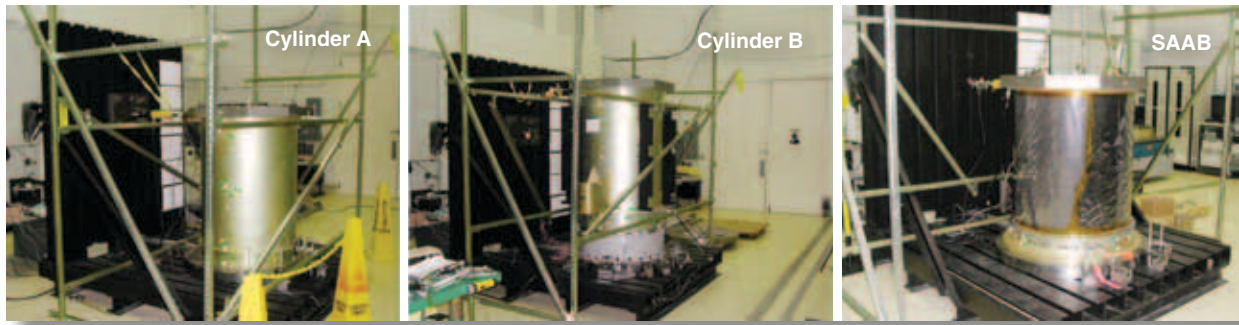
Figure 7. Static load test configurations.
