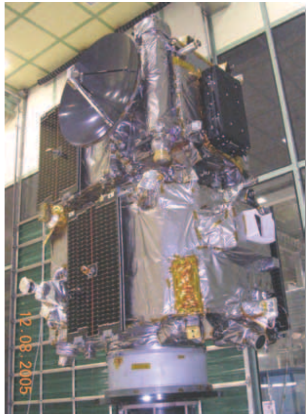
Figure 23. Stacked STEREO observatories, spin balance and vertical mass properties configuration with water-filled tanks.
