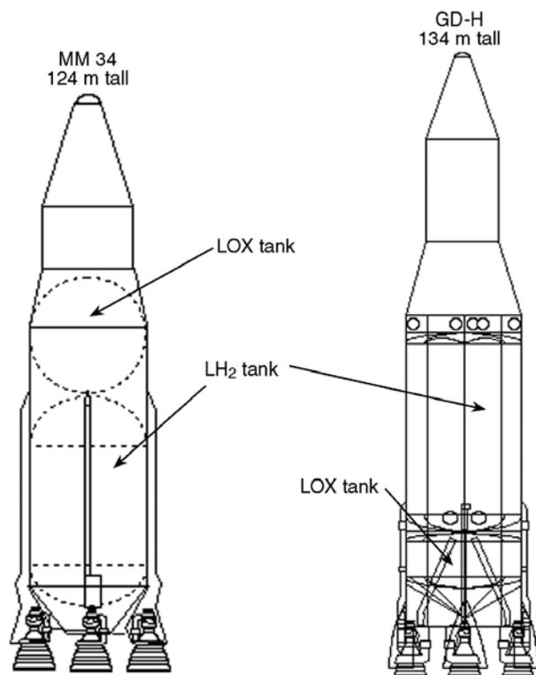
**Figure 1.** Two scalable Nova concepts from the 1960s using 1.5-stage LOX/LH<sub>2</sub> systems. Details about these and other designs are discussed later in this article. (Reproduced, with permission: © Mark Wade; <http://www.astronautix.com/>.)
