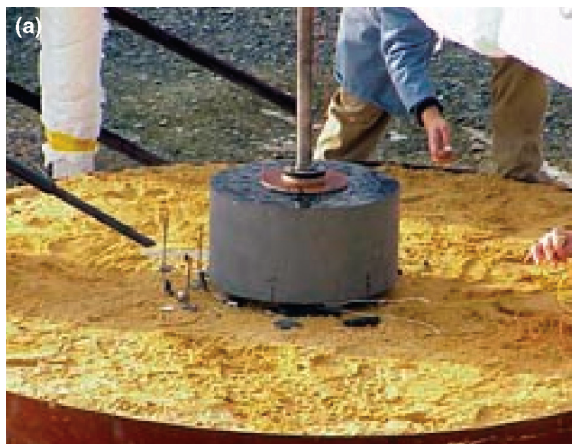
Figure 3. (a) Test setup with propellant block and in situ instrumentation. (b) LWIR image of a solid propellant fire test.
