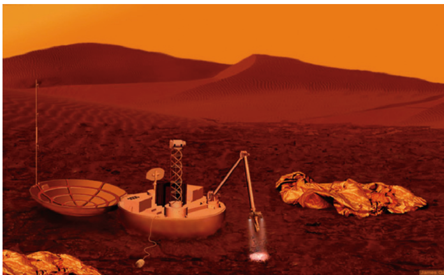
Figure 9. Artist's impression of a lander sitting amid Titan's dune fields. The sampling arm is equipped with a UV lamp to excite fluorescence in specific organic compounds. A seismometer/magnetometer package lies in the foreground, connected to the lander by a tether, and a meteorology mast is at left. (Artwork by James Garry [www.fastlight.co.uk]; used with permission.)
