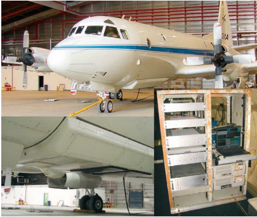
Figure 3. D2P installation on the NASA P-3 aircraft: (clockwise from top) aircraft, D2P equipment racks, and bomb bay-mounted antenna.
