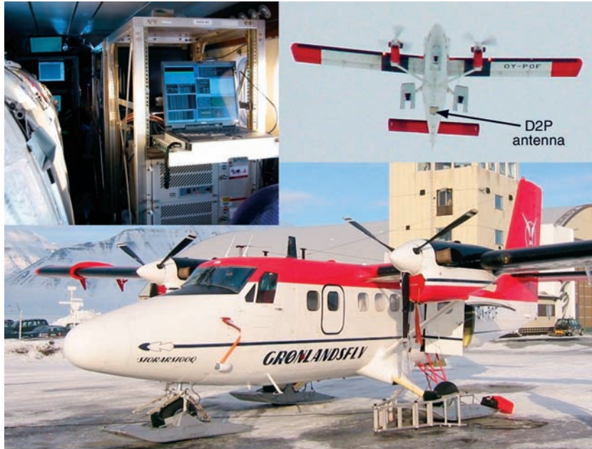
Figure 5. D2P installation on the Greenland Air Twin Otter aircraft: (clockwise from bottom) aircraft, D2P equipment racks, and bottom view of aircraft showing the antenna just aft of the rear wheels.
